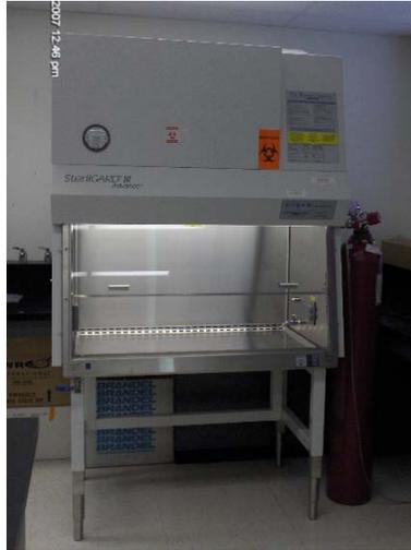
**Figure 5.2.** Biological safety cabinet. Example here is a class II-A cabinet which does not have a hard ducted exhaust system. The front sash has an optimal height setting to minimize disruption of the protective air curtain at the front of the work area. Moving the sash higher than this optimum setting will cause the cabinet to alarm.
