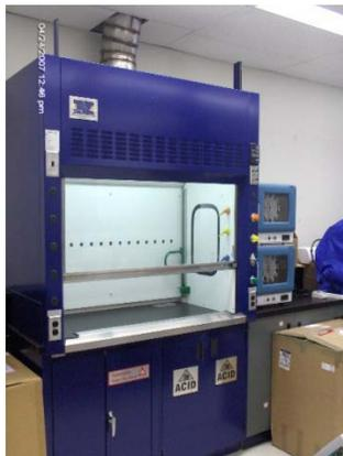
**Figure 5-4.** Chemical fume hood. Note the hard ducted exhaust vent leading from the back of the fumehood into the room ceiling. The height of the front sash is adjustable, however the higher the sash is raised, the more likely the protective air flow at the front of the work area will be disrupted by passing traffic.
