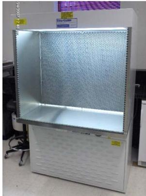
**Figure 5-3.** Laminar flow hood. Note the lack of a protective sash across the front. The back wall of the flowhood is a HEPA filter system. The clean filtered air is blown across the work surface and out towards the user and room. Aerosols generated from the product will be blown into the face of the user and dispersed into the laboratory.
