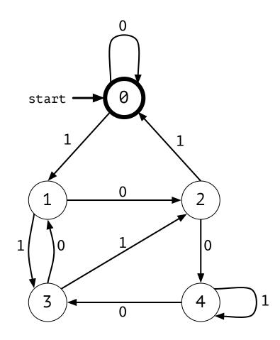
d) [3 marks] Draw a FSM from the description that accepts precisely binary numbers that are divisible by  $3_{10}$  and either are the number zero or have a leading 1. Example: 11 and 0 are accepted; 011, 00, 10 are rejected.
