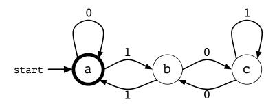
Figure 1: A finite state machine that accepts binary numbers divisible by 3. Here, **a** is both the start state and the accepting state.
